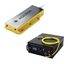
The FCMH series diode lasers deliver up to 500 W of power through a 200 µm fiber. They provide high brightness and simplified thermal management by distributing the diodes (heat sources), allowing for a water-cooled architecture with reliable, predictable performance. A turn-key benchtop unit is available, integrating the power supply, water cooling, power control, and safety shut-off features.
